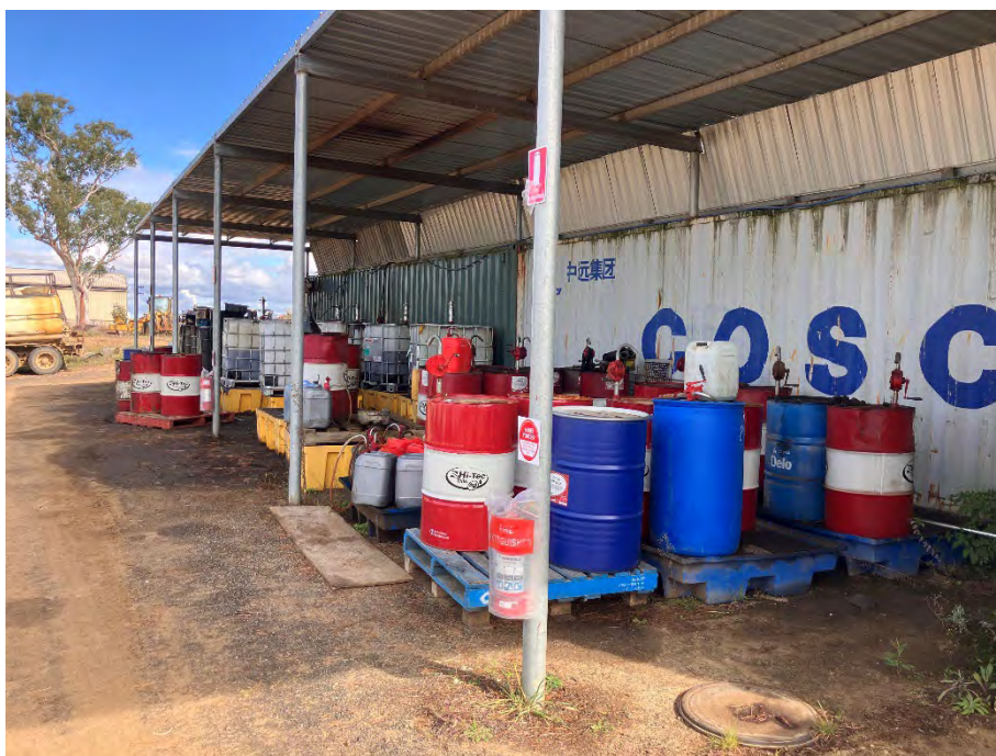
Photo 15: Lubricant storage at maintenance workshop with most items stored on portable bunds, however some soil staining evident, looking south.
